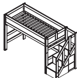
LOW-LOFT BED WITH STEPLADDER H 152 x W 257 x D 102 Ground clearance below the bed 113 CM
